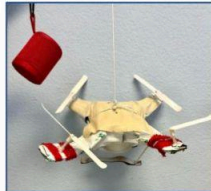
Dummy drone, and speaker playing drone sound
