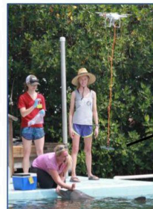
Flying the drone over DRC dolphins comfortable with it and asking them to chuff helped refine the petri dish array and determine optimal height of the drone
